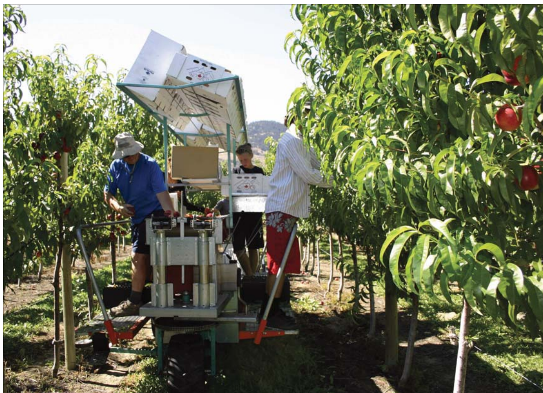
Figure 1. Harry Shaw, left, places peaches on the central conveyer belt. He and a hired helper, Nathan, are standing on the platforms on either side of the harvester while Starr Shaw is at the back sorting fruit. Boxes are kept on the superstructure until needed. An arm with a sensor (small wheel) at the end which can be seen in the lower left of the photograph allows the harvester to be self-steering.
